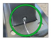
Pin must be fully inserted through the lock tab while carrying or using the Sharks™. Only remove pin during opening or collapsing of the Sharks™ and reinsert the pin prior to moving, carrying or applying load to the Sharks™. Never move or use a Shark™ without the pin fully inserted through the lock tab.
