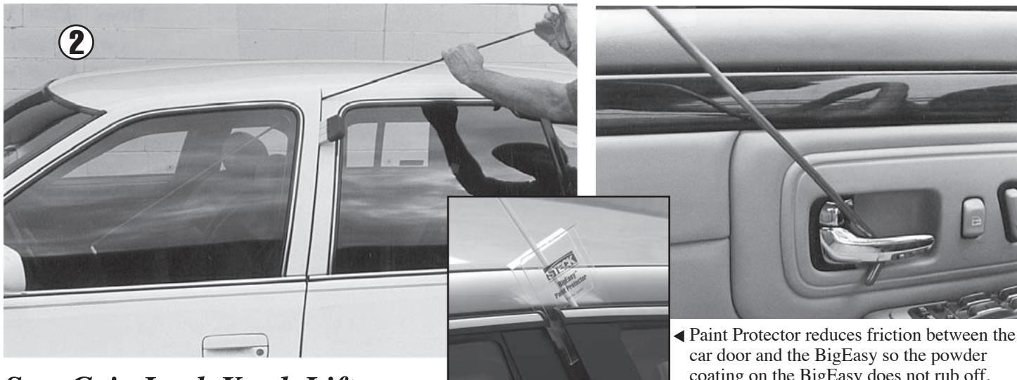
◀ Paint Protector reduces friction between the car door and the BigEasy so the powder coating on the BigEasy does not rub off.
