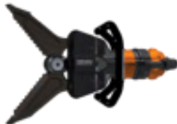
CT 5114 ST Spread: 303,492 lbf Cut: 60,249 lbf 14.3" · 20.1 lbs.
