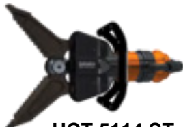
HCT 5114 ST Spread: 303,492 lbf Cut: 60,249 lbf 14.3" / 20.1 lbs.
